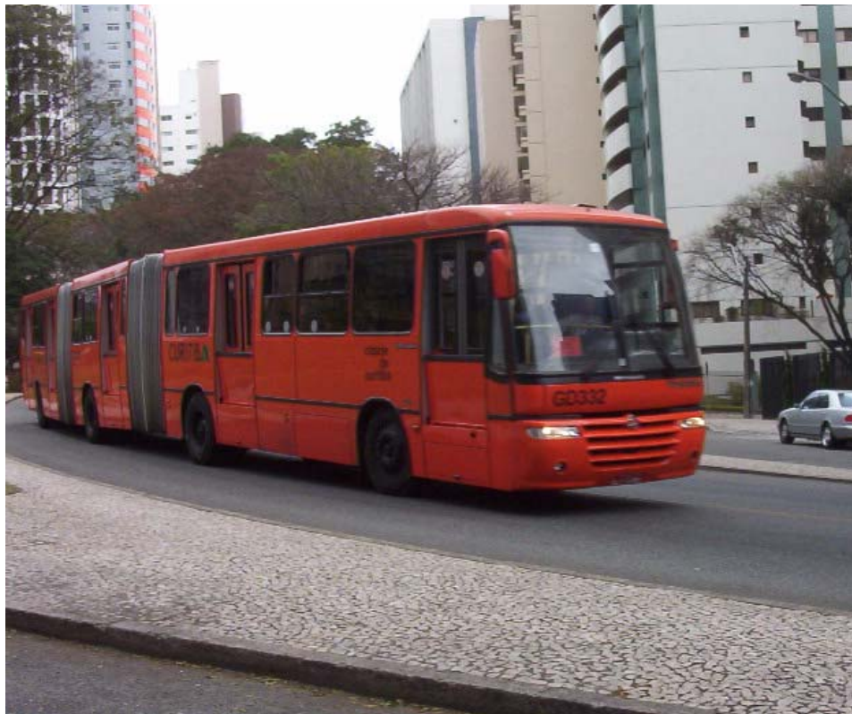
Bi-articulated Bus on South Busway
